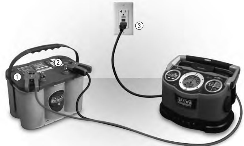
Pictured: Typical DC charging clamp connections for a precharge status, charging or just maintaining a fully charged battery with the DC charging clamps out of vehicle.
